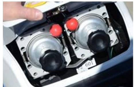
For the trial, employees at the exchange stations performed the canister switch but switching is a simple process that can easily be done by the driver.
